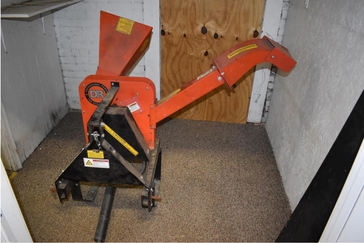
DR Field and Brush Chipper – 3 Point PTO Drive
